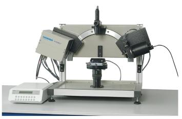
Fig.2: UVISEL with temperature cell
