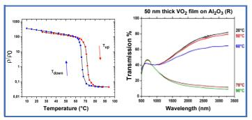
Fig.1: VO<sub>2</sub> SMT transition: electrical (left) and optical (right) properties
