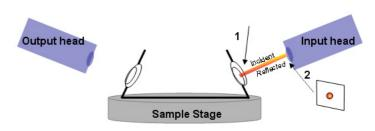
Fig.3: Schematic - positioning the temperature cell
