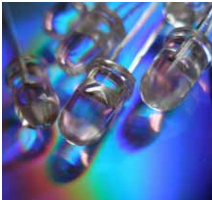
Figure 1b, An image of a packaged deep UV LED
