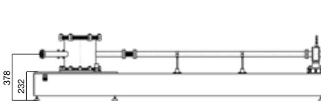
TGM1900 in HV version, with two gratings in slider, custom version without entrance slit and arm
