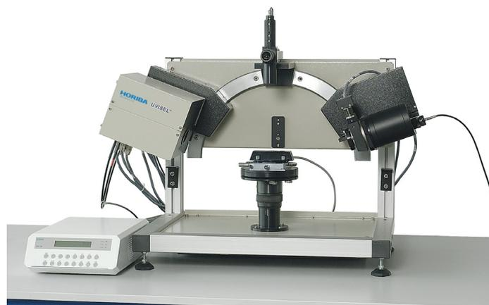
Fig.2: UVISEL with temperature cell
