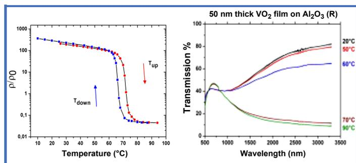
Fig.1: VO<sub>2</sub> SMT transition: electrical (left) and optical (right) properties
