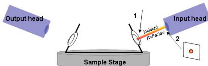
Fig.3: Schematic - positioning the temperature cell
