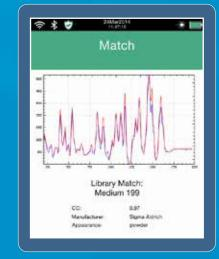
Many common materials can be measured and detected by Raman handheld instruments. Metals, salts, and some packaging materials still represent a challenge to any type of Raman technology. Talk to your Rigaku Raman representative about your list of raw materials.
