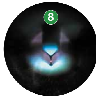
Visual confirmation of Raman laser alignment in all modes
