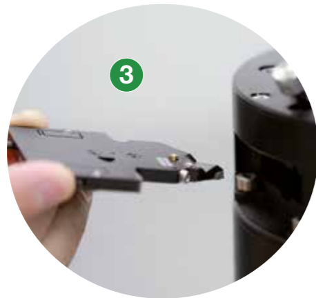
Compact holder for easy probe exchange
