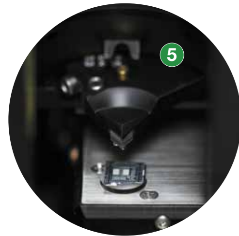
High resonance scanner, auto tip-alignment and tuning
