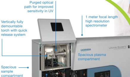
Built-in 3 channels peristaltic pump and external sample introduction system for facilitated access
