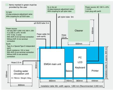
\*Please note that the indicated lengths of tubes, power cables, etc., are based on the length of accessories included. In the actua installation, ensure that the layout allows for some freedom of movement.
