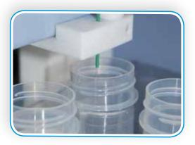
4. <u>Sample Handler</u>: Once digestion is complete, return the rack with samples to the **Sample**Handler. Add internal standard directly into each sample *Digi*TUBE.
