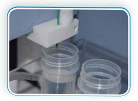
Sample Handler: Transfer samples from the 50 ml *Digi*TUBE rack to a 15 ml autosampler tube rack. Analyze by ICP or AA.
