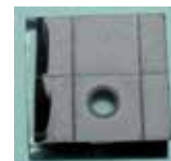
Analysis time - 2 min, crater diameter - 4 mm.
